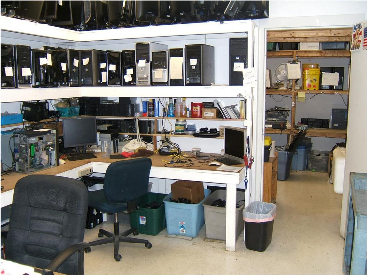
Disassemble PCs and other equipment we cannot use, and separate the parts into bins of copper, aluminum, etc. for sale to scrap dealers. Again, all done by volunteer members. We strip the PCs in the room shown past the door to the right above.
